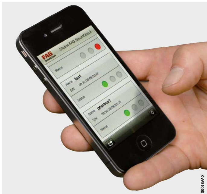
Figure 2 Smartphone as alarm receiver
